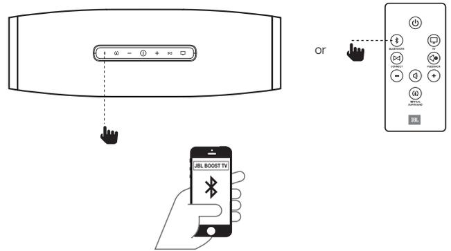
1. Press the Bluetooth button on the top-panel or remote control. The button light will blink slowly, indicating that there is no connected Bluetooth device. If you have never paired a Bluetooth device before, the JBL BOOST TV will enter pairing mode directly, which is indicated by the button light fast blinking. Skip step 2 for the first time you pair a Bluetooth device.
